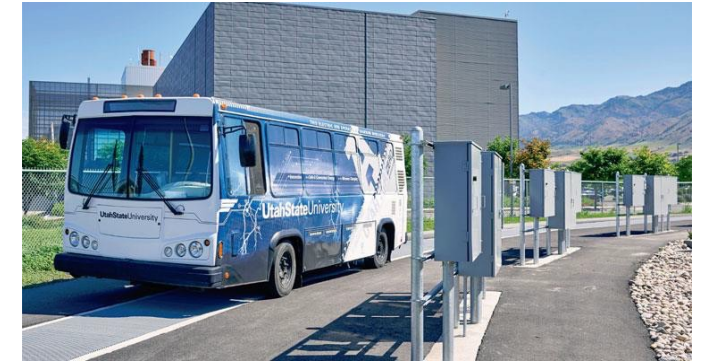
In-motion wireless charging and autonomous control of the “Aggie Bus” on the EVR track
